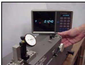
TF-IND Fixture Positions AGD and ISO Indicators for Calibration
