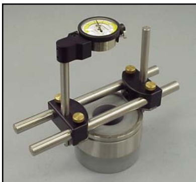
Round standards set the distance between the thread shoes on the MRP gages
