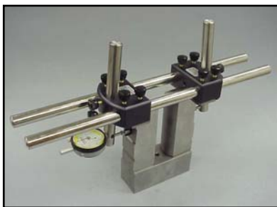
Frame standards set the distance between the thread shoes on the MRP gages
